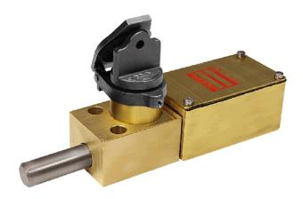
Type S auxiliary switches are slow-make, slow-break devices that respond directly to the movement of the lock bolt when the key is rotated. One, two, three or four sets of contacts are available. The Type S auxiliary switches can be furnished on the following interlocks:
